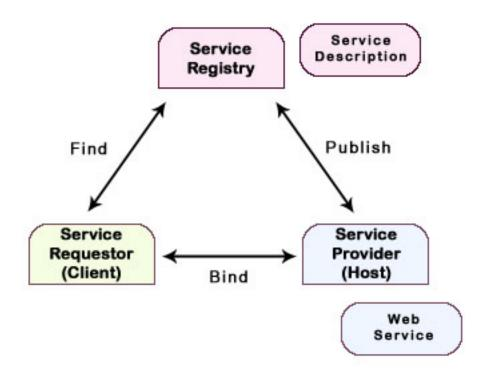
In the above figure "Service Requester" acts as client of the web service and the "Service Provider" as host of the web service. Client makes a request for the web service to the provider and provider sends response accordingly.
